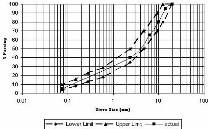
Figure 1. The Grading Curve of Asphalt concrete.
