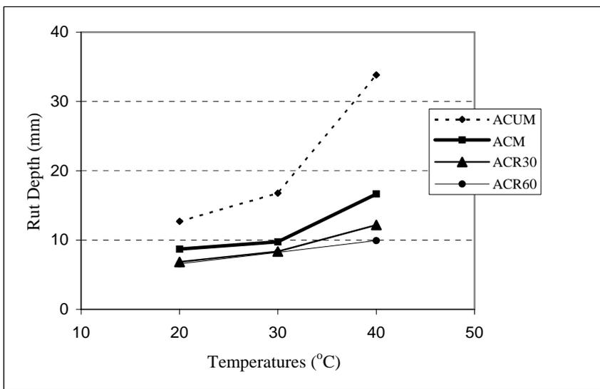
Figure 10. Prediction of Rut Depth Using VESYS 5 at 10<sup>th</sup> Year Under Varying Temperatures.
