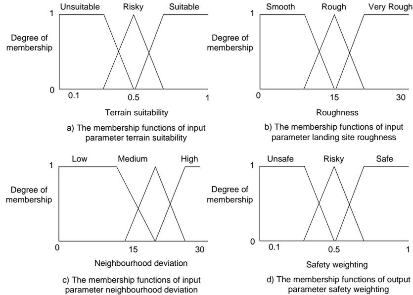
**Fig. 3.** The membership functions of fuzzy logic parameters
