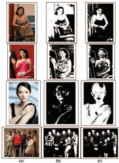
Fig. 6. columns (a), (b) and (c) represent random images from google, skin segmentation using Cheddad et al. [4] and our methods respectively.
