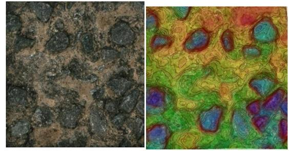
Figure 10: Image and corresponding model of 14mm single sized surface dressing
