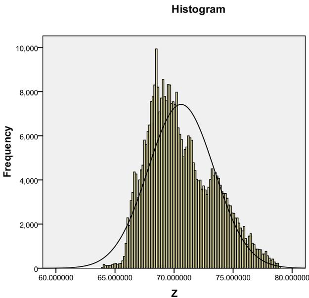
Figure 9: Frequency distribution for heavily trafficked 14mm single size surface dressing
