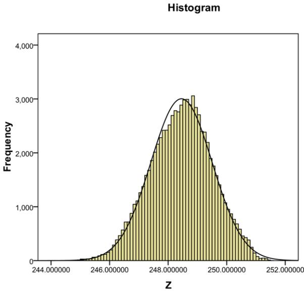
Figure 8: Frequency distribution for 14mm/6mm surface dressing
