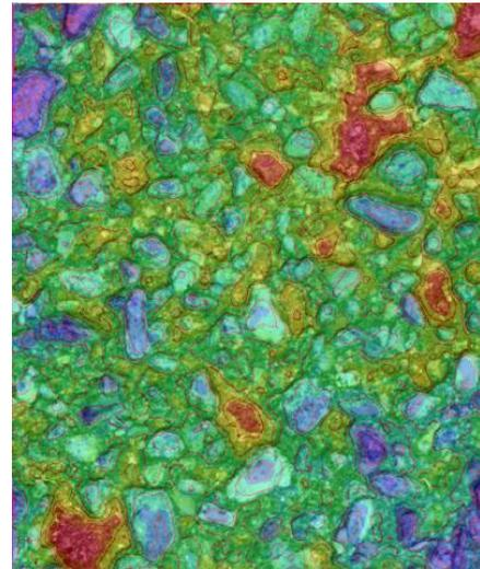
Figure 6: Depth banded model of 14mm/6mm surface dressing
