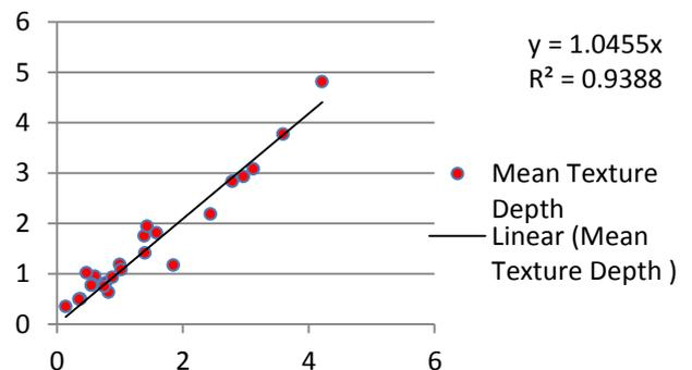
Figure 7: Correlation of MTD estimated by sand patch and DEM
