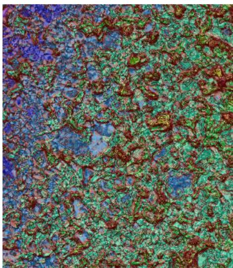
Figure 5: Depth banded model of 10mm asphalt concrete
