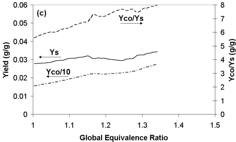
Fig. 4. The smoke and CO yields together with the ratio  $Y_{co}/Y_s$  as a function of the GER. Fuel: propane.
