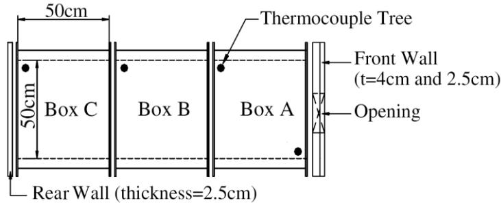
Fig. 1. Top view of the experimental compartment.
