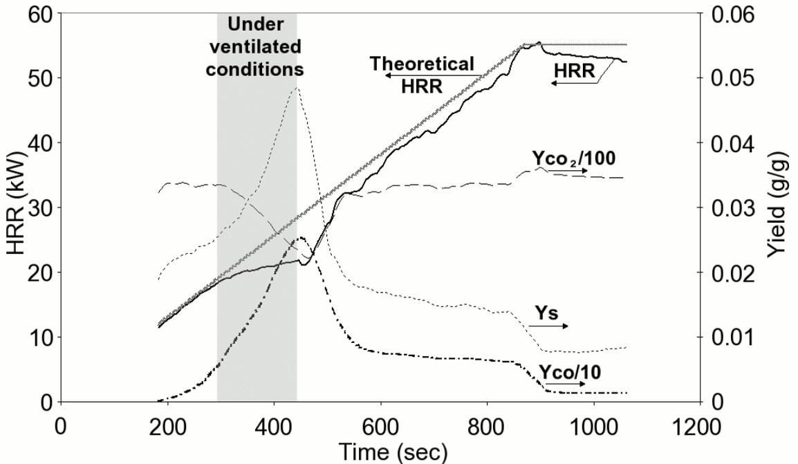
Fig. 3. Heat Release Rate together with the smoke, CO and CO<sub>2</sub> yield. Fuel: propane. Opening size 0.1m\*0.25m. 1 box geometry.
