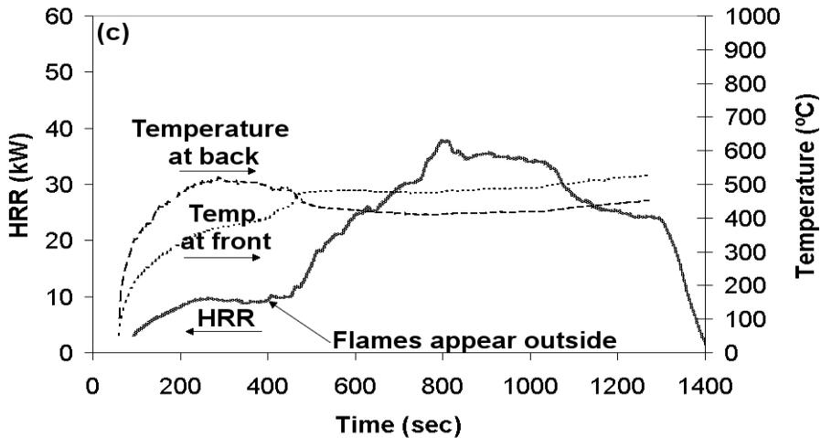
Fig. 5. Upper layer temperature together with HRR. 2 boxes geometry. Fuel: propane.
