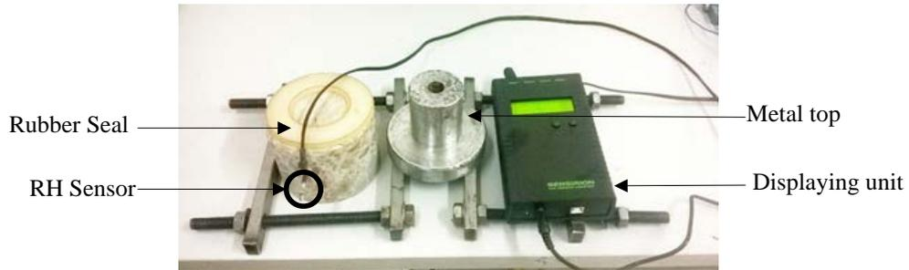
**Figure 2** The probe of measuring RH at surface and in the drilled cavities
