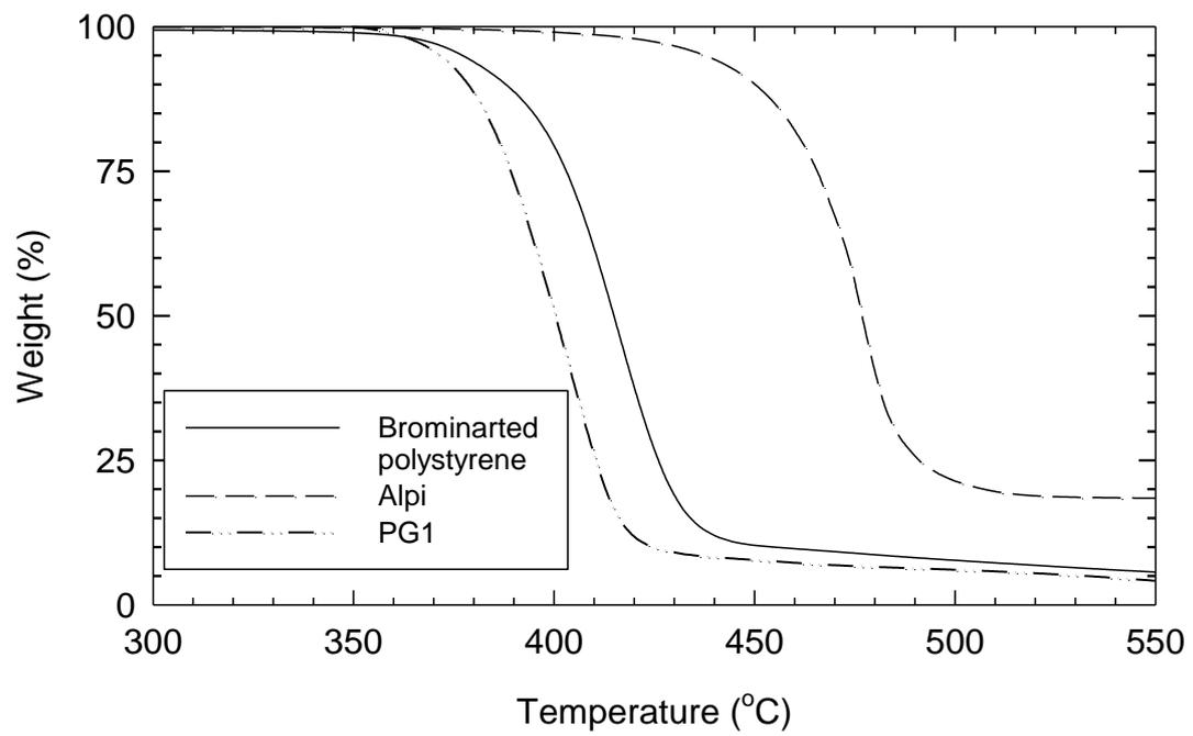
Figure 3. TGA curves of brominated polystyrene and Alpi (PG1 as reference).
