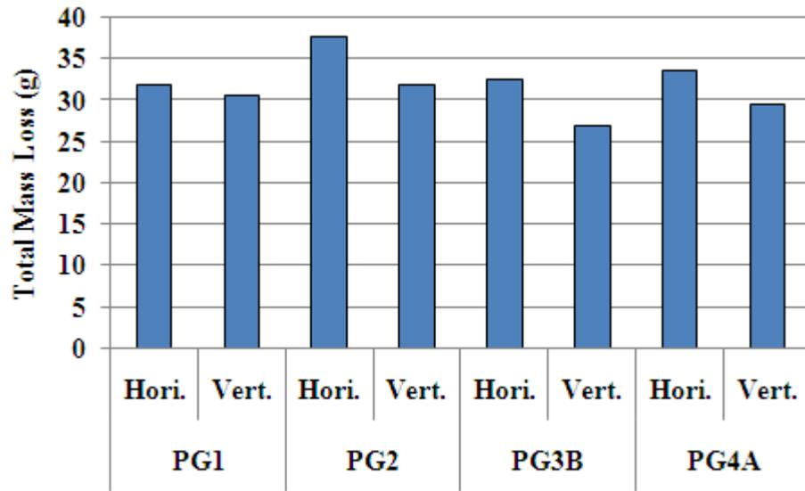
Figure 13. Comparison of total mass loss (g) between horizontal and vertical tests.
