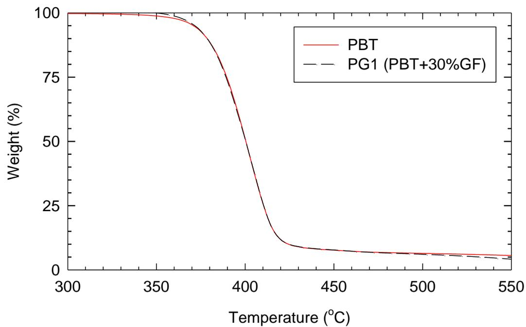
Figure 1. Comparison of the mass loss (TGA) curves between pure PBT and glass-fibre enforced PBT (PG1) at 10 °C/min in nitrogen. The weight of PG1 was normalised by the initial weight of PBT in PG1.
