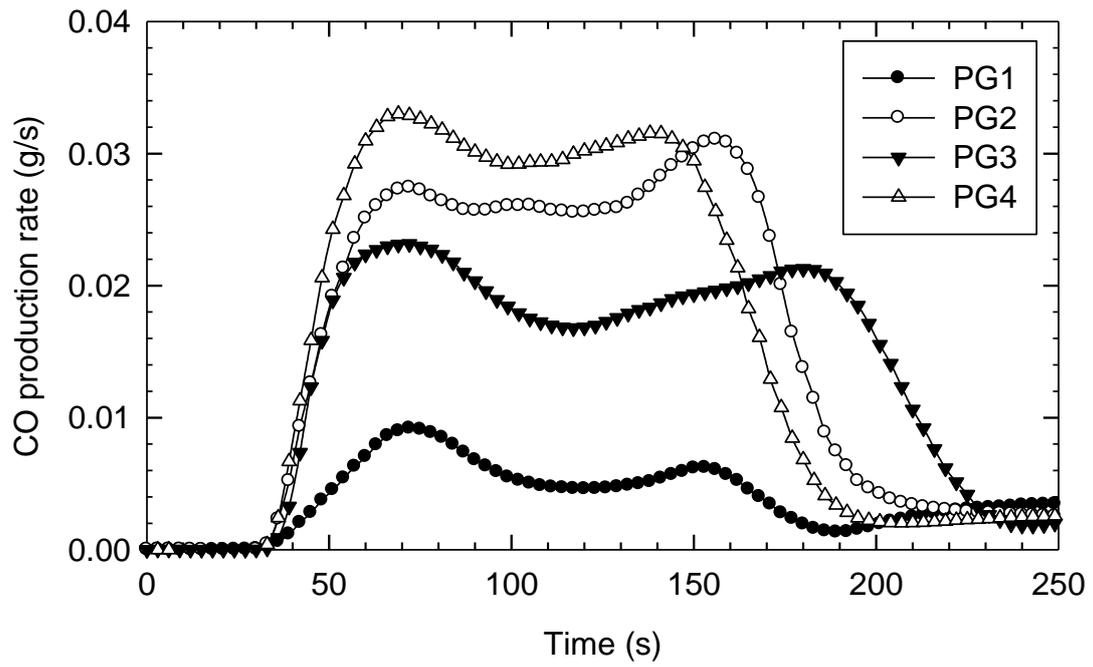
Figure 7. CO production rate (g/s) at 60kW/m<sup>2</sup> in the horizontal cone calorimeter.
