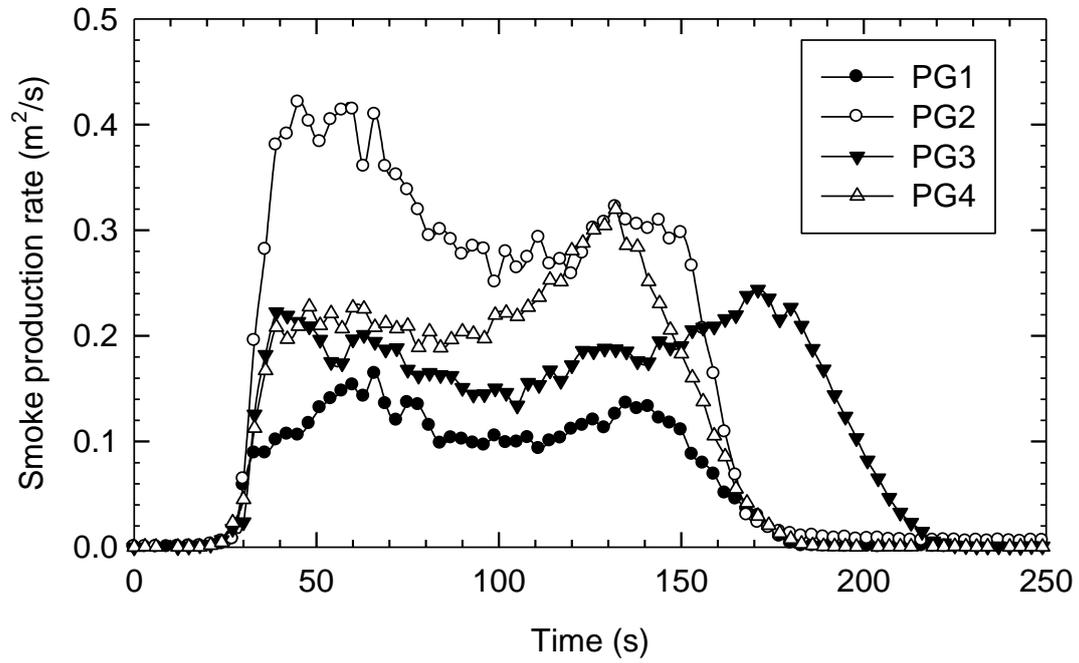
Figure 8. Smoke production rate ( $\text{m}^2/\text{s}$ ) at  $60\text{kW}/\text{m}^2$  in the horizontal cone calorimeter.
