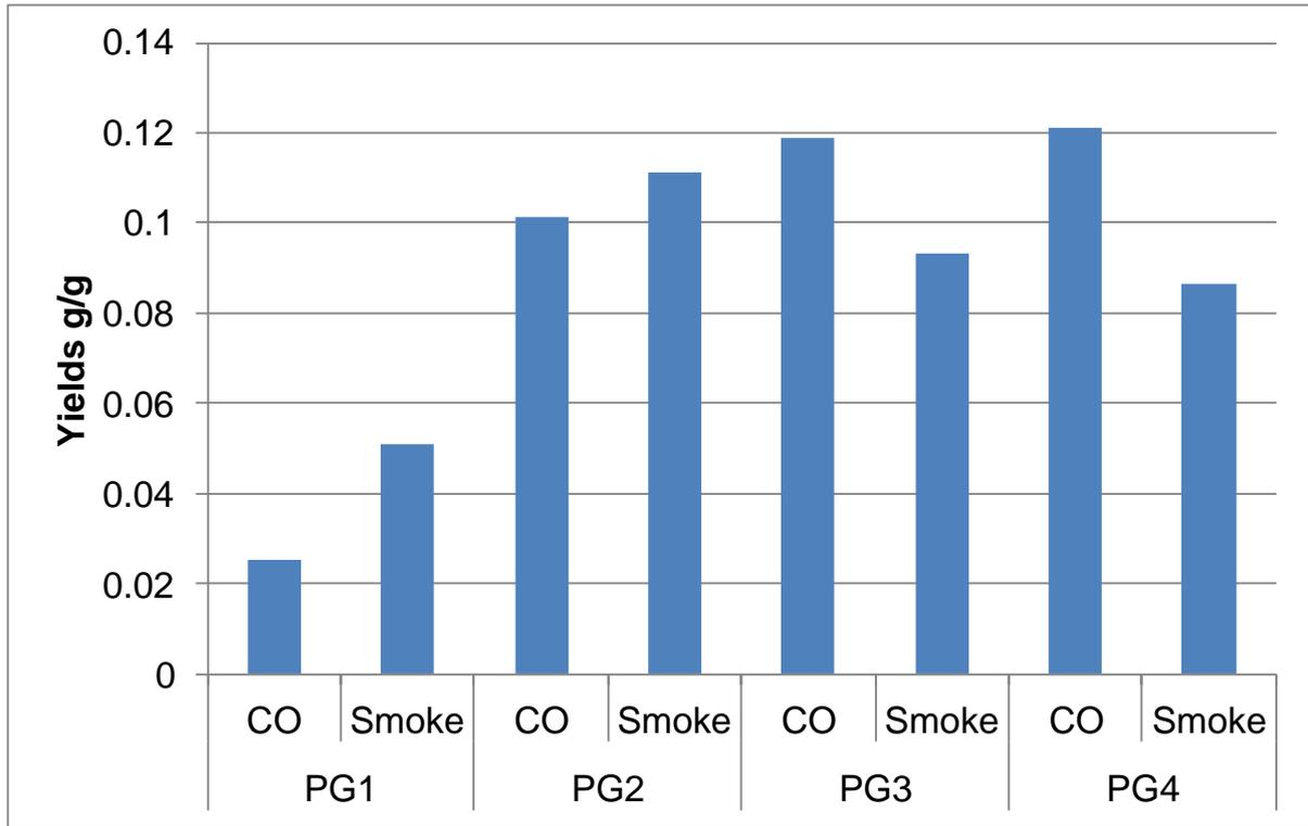
Figure 9. Average CO and smoke yields at all heat fluxes in the horizontal cone calorimeter.
