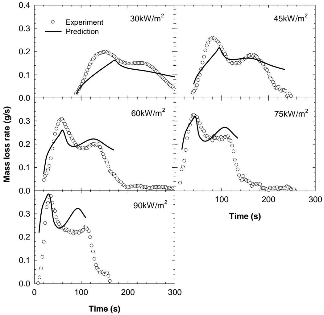
Figure 11. Comparisons of experimental and predicted mass loss rates of PG1 at different heat fluxes.
