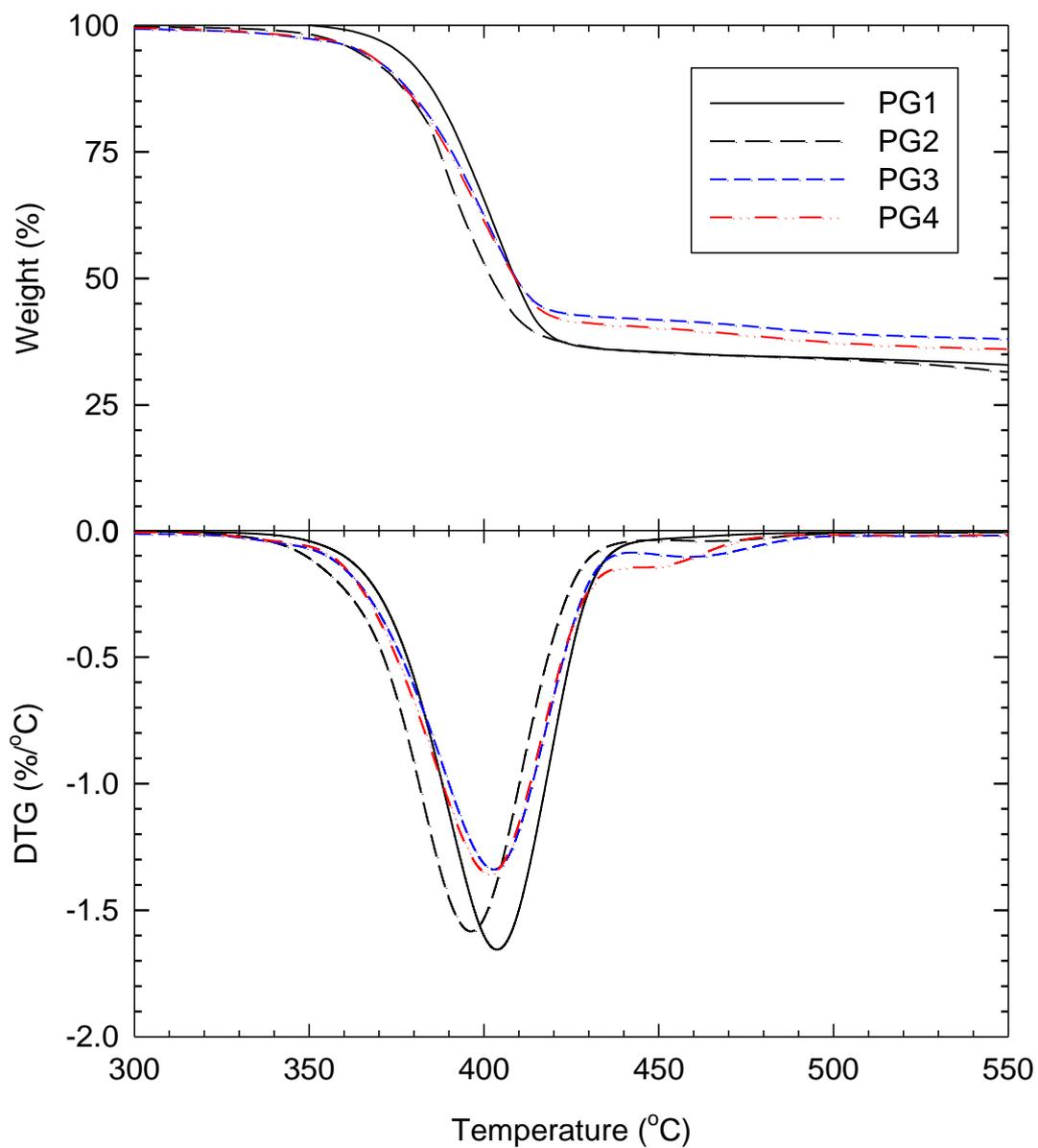
Figure 2. TGA and DTG curves at 10 °C/min in nitrogen.
