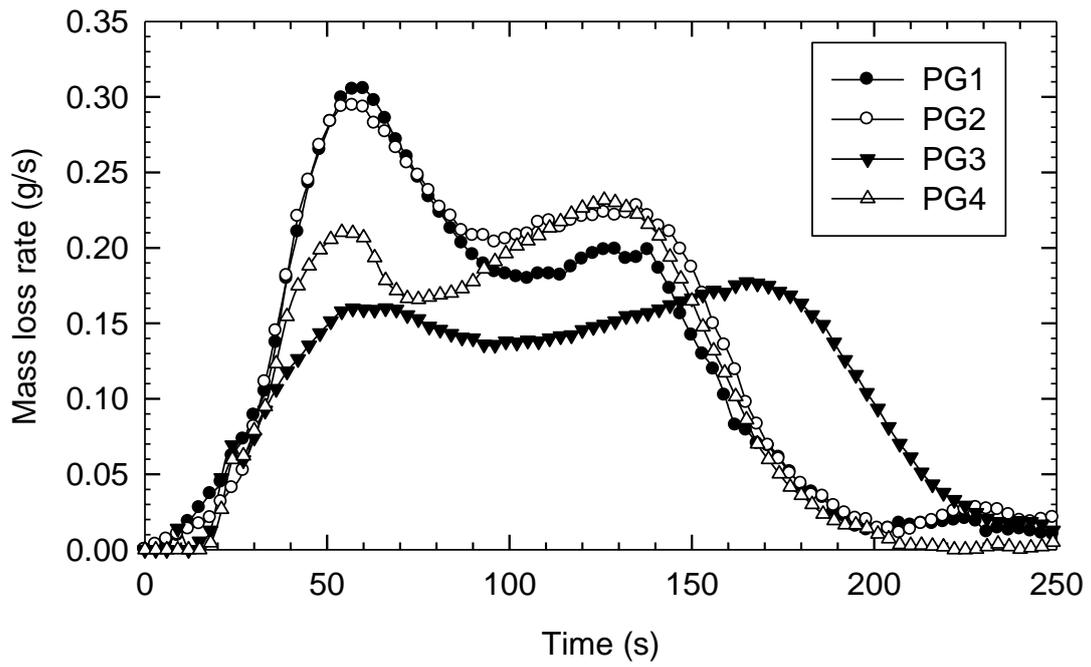
Figure 4. Mass loss rate at  $60\text{kW/m}^2$  in the horizontal cone calorimeter.
