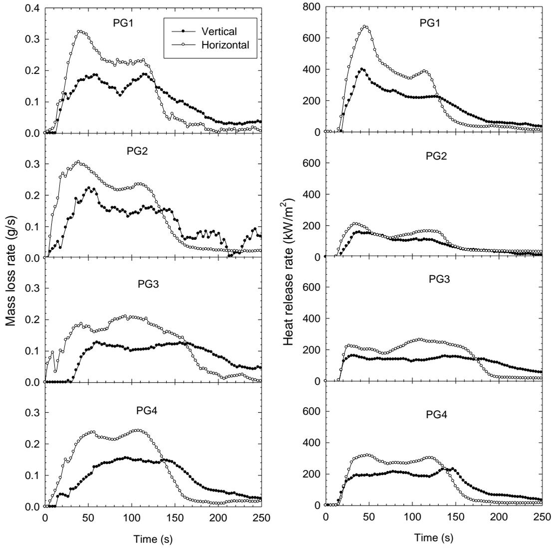
Figure 12. Comparison of MLRs and HRRs at 75kW/m<sup>2</sup> between horizontal and vertical tests.
