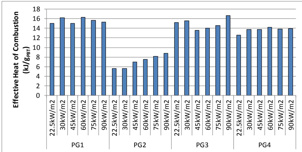
Figure 6. Comparison of effective heat of combustion (kJ/g<sub>PBT</sub>), calculated by dividing the total heat released by the PBT content in each formulation, in the horizontal cone calorimeter.
