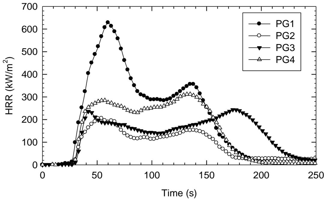
Figure 5. Heat release rate at 60kW/m<sup>2</sup> in the horizontal cone calorimeter.
