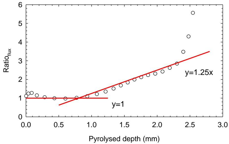
Figure 10. Calculated instantaneous heat flux ratio,  $ratio_{flux}$ , against the pyrolysed depth,  $\delta_{pyro}$ , at  $60 \text{ kW/m}^2$  (sample thickness is  $2.9 \text{ mm}$ ). Two lines represent the best fits of the calculated results.
