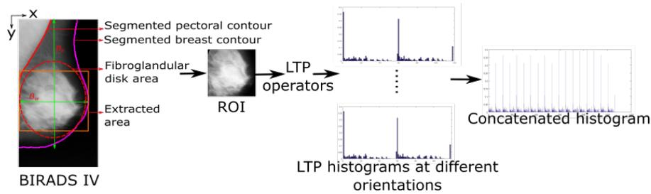
Fig. 3. Summary of feature extraction in our study using the LTP operators.
