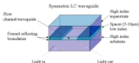
**Figure 1:** Leaky Waveguide Device with integrated micro-flow channel
