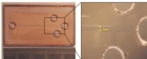
**Figure 5:** Liquid Photoresist chip.
