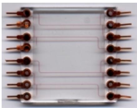
**Figure 4:** The Injection moulded separation device, with integrated electrodes.
