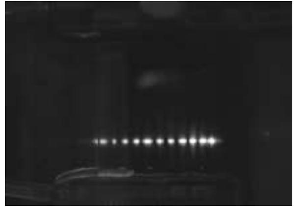
**Figure 5.** Ten channel laminar flow system using orthogonal Leaky Wave excitation of fluorescence at 473 nm
